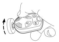
Likewise, when rotating the IKT to the off position in the ignition lock cylinder, the bottom edge of the IKT adjacent to the control can be utilized.
